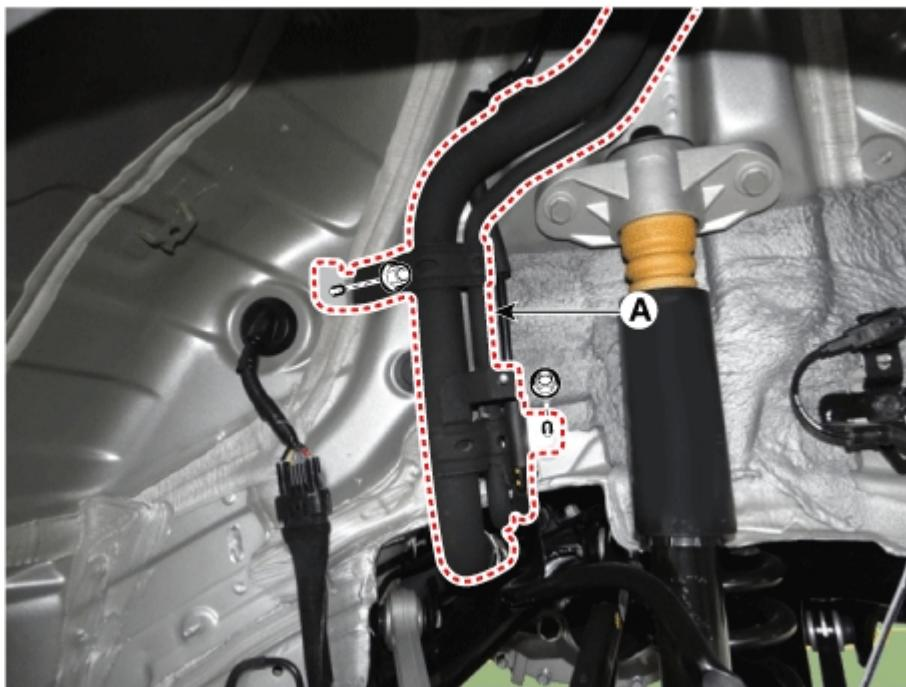
5. After loosening the mounting bolts, remove the fuel filler door (A).
