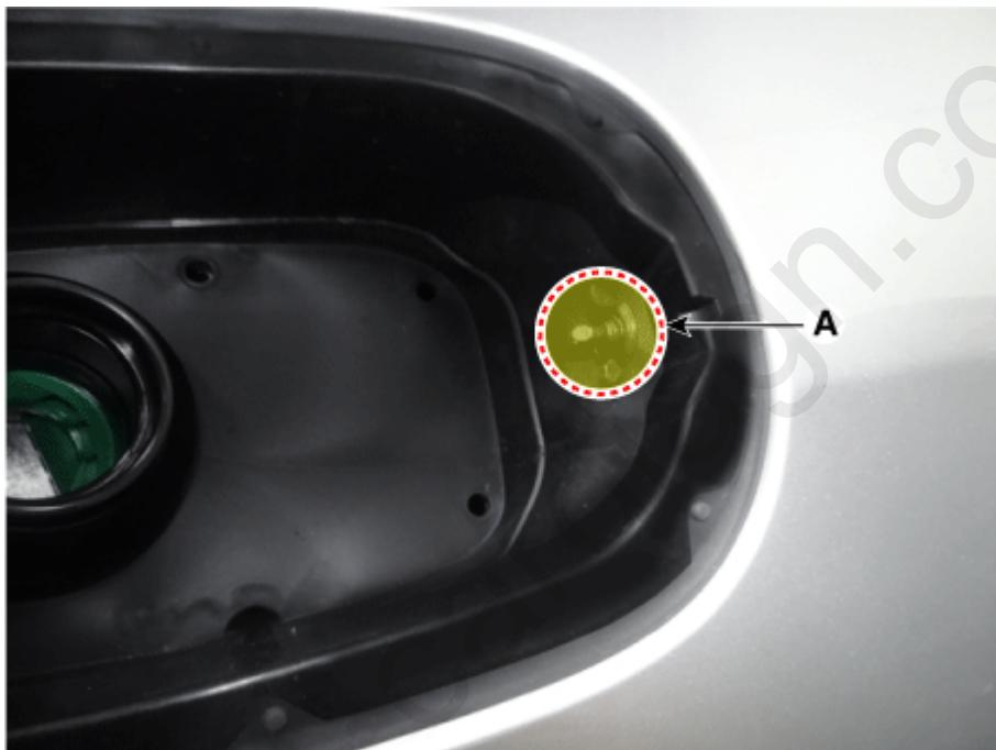
4. Separate the filler neck (A) after loosening the mounting nuts.
